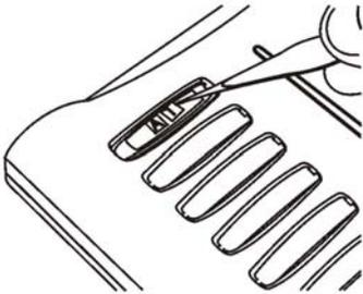
3. Then install button casing back on the main board.
